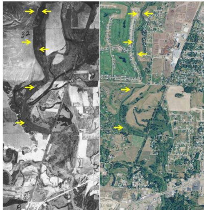
Figure 61. Aerial photographs of the Whitefish River near the mouth in 1936 (left image) and 2009 (right image). Yellow arrows indicate areas where riparian vegetation has been removed and currently provides less shade than in the past.
